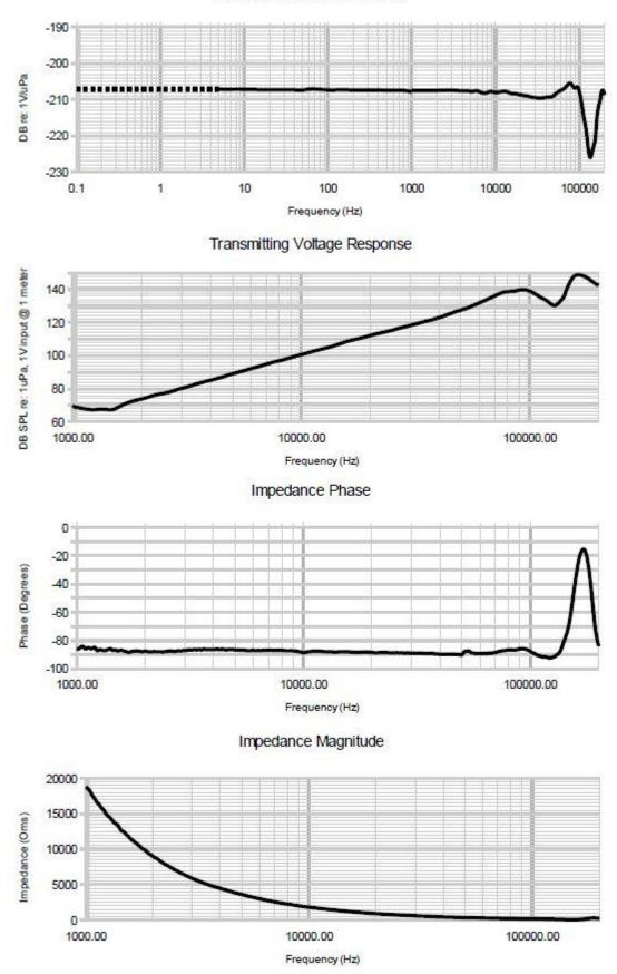
FFVS: Nominal 5Hz - 100KHz, -207.6 (+2.1 / -2.0) dB re: 1V/uPa. Not tested (theoretical) below 5Hz.
